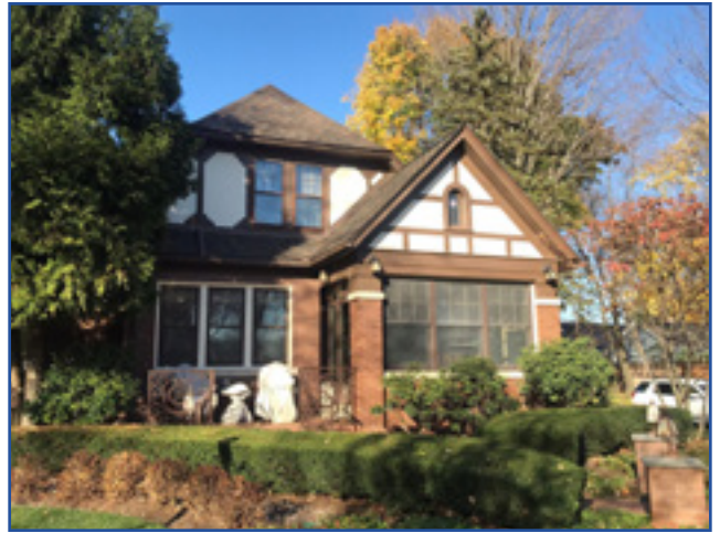
Tudor Revival house with a prominent, front-facing gable and decorative half-timbering. City of Birmingham, photo by KDG, 2022.
