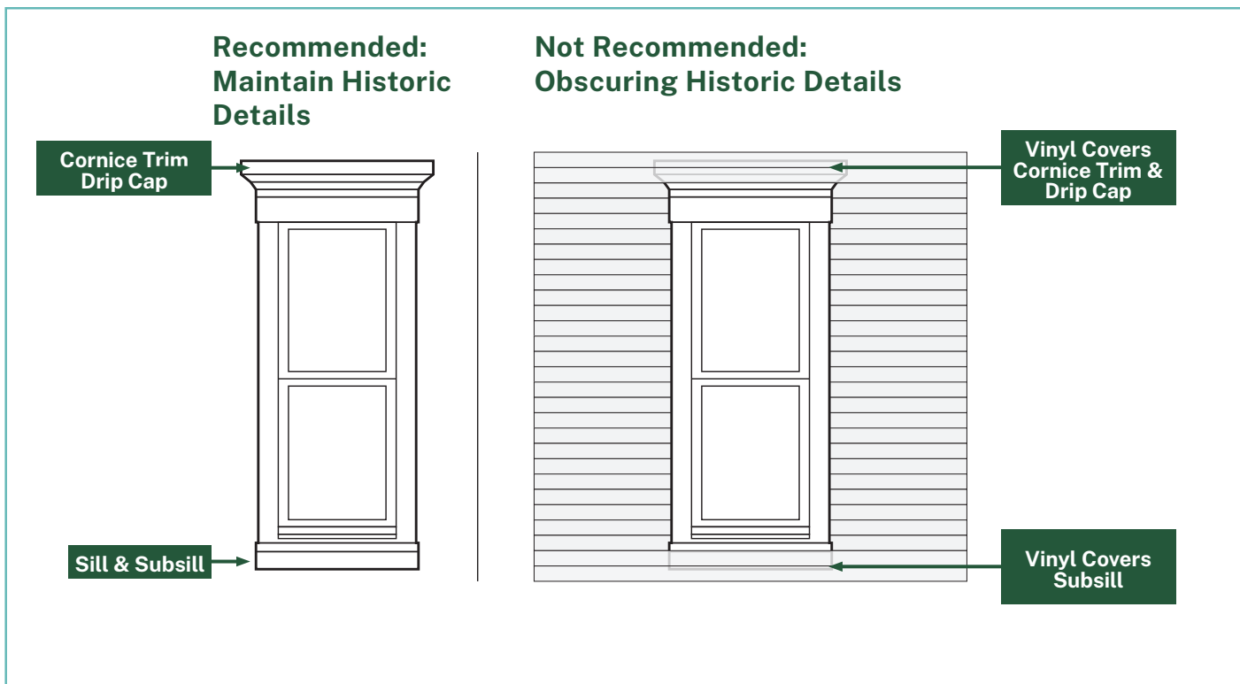
Installation of modern siding often obscures or results in the removal of character defining details.
