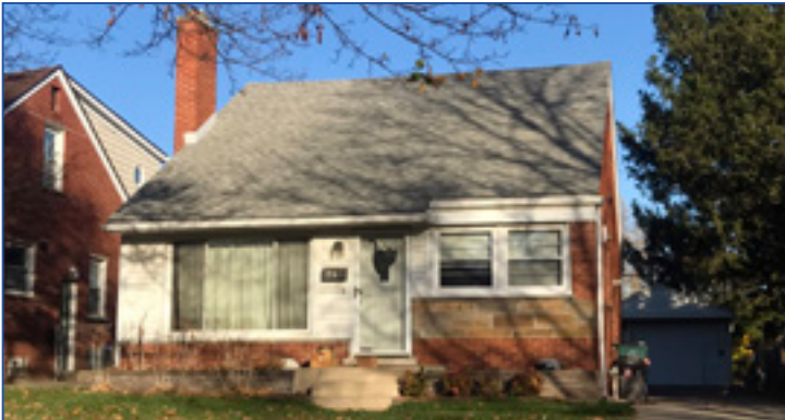
Small houses with minimal decoration and side gable roofs are indicative of the Minimal Traditional style. Brick and stone veneer and siding are incorporated into the exterior cladding on this example. City of Birmingham, photo by KDG, 2022.
