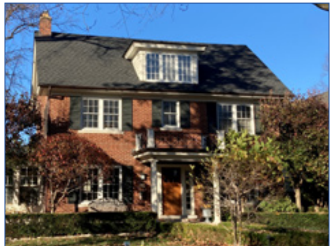
The paired, 6-over-6 windows, shutters, portico, symmetrical façade, and side gable roof are indicative of the style. City of Birmingham, photo by KDG, 2022.
