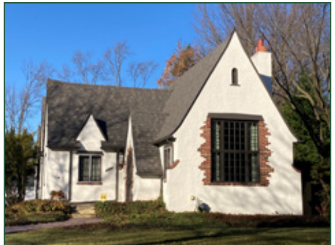
A stucco exterior clads this Tudor Revival with a large, front-facing gable and brick accents around window and door openings. City of Birmingham, photo by KDG, 2022.
