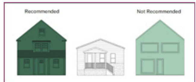
Construction of the new home at right would not be recommended in a historic district containing modestly scaled homes, as shown at left. The scale of the new construction overwhelms neighboring homes. City of Birmingham, photo by KDG, 2022.
